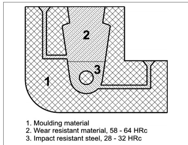
Figure 2. Principle of molding bimetallic hammers [7]
