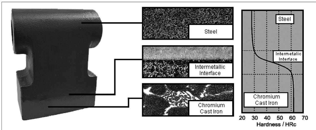
Figure 3. Metallurgy and hardness of bimetallic hammer castings [7]
